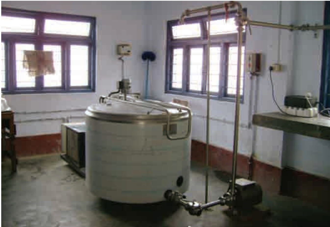
Picture 2: Bulk milk cooling machines installed at a Village Milk Cooperative Society to arrest bacterial growth
